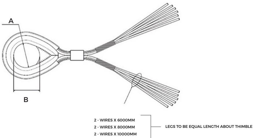
Wire Rope Ø8mm, 6 X 19 Fc galvanised ends tapered and fused.
