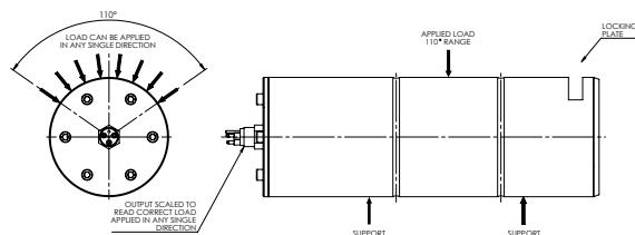
For a given load applied in any single direction within the load application region, the Force Magnitude Shear Pin Load Cell will output a consistent calibrated 4-20mA output where 4mA=0t and 20mA = WLL, or R485 MODBUS output. This removes the need to have a load direction on the Shear Pin Load Cell and allows for use in application with a varying load direction.
